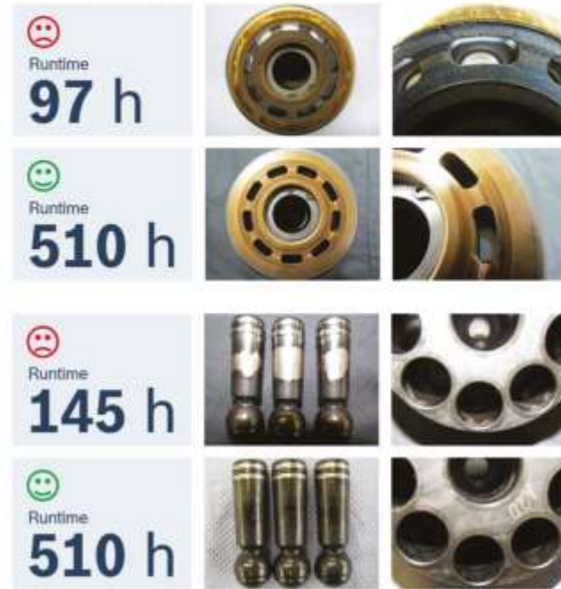
Figure 6a+b. On the one hand, Bosch Rexroth tests show fluids that have led to significant damage after fewer than 100 operating hours. Other hydraulic fluids cause no wear whatsoever after 510 hours. (Copyright: Bosch Rexroth AG).
